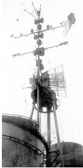
Fig. 2.19 The light cruiser Scipione Africano with the antennas of the RDT E.C.3-ter “Gufo”. The position of the antennas allows us to distinguish, at the rear, the rudder added to compensate for the insufficient power of the electric motor in the presence of wind
