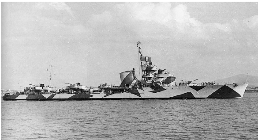
Fig. 2.35 The destroyer Legionario , first Italian unit equipped with an operational radar, photographed on May 18th, 1942. The antenna of the German radar “De Te” type FuMO 21/40 G is visible, after its installation in March 1942
