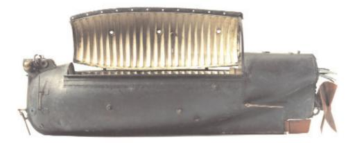
Fig 1 : Wilhelm Bauers functional model of a submarine, the upper watertight service hatch is lifted open
