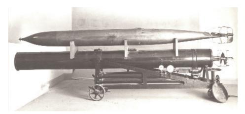
Fig 5: Torpedo C/84A, on top of a lancing tube (built by Whitehead, date unknown) with Torpedo C 77.<sup>11</sup>
