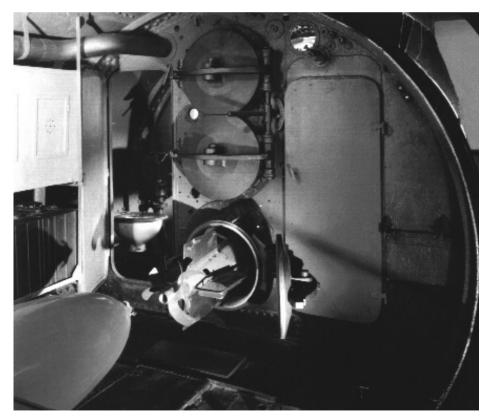
Fig 6: Torpedotubes in the submarine "U 1", 1906. One tube was used for lancing, the other two were kept for the storage of torpedos of the C03 type.<sup>12</sup>
